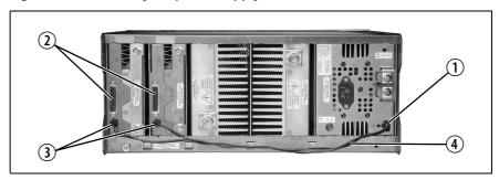
Two different types of auxiliary DC output connector have been fitted to the PMU. The pin allocations for the 8-way connector fitted to PMUs manufactured before August 2004 are given in the following table. Note that pins 1 to 4 and pins 5 to 8 on this connector are linked.
