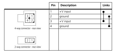
The DC output from the PMU is 13.65 VDC, 27.3 VDC, or 54.6 VDC (depending on the model). Although this power output is isolated, the negative side of the supply is grounded on the system interface board to give a +V output.
